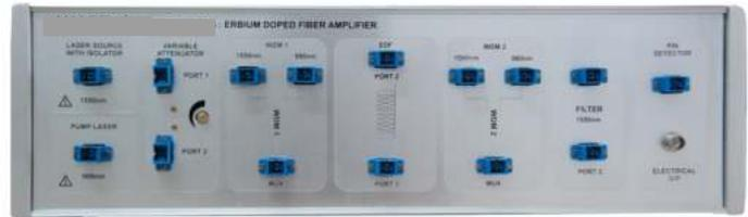
Bench top EDFA training system is designed to understand the principles of Optical Amplification and provides hands-on experience in building Erbium Doped Amplifier. This system enables the student to measure the optical amplifier characteristics under forward and backward pumping schemes.
